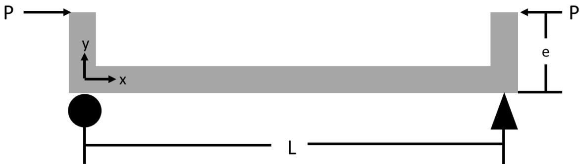
Figure 1: Simply supported beam buckling with eccentricity
