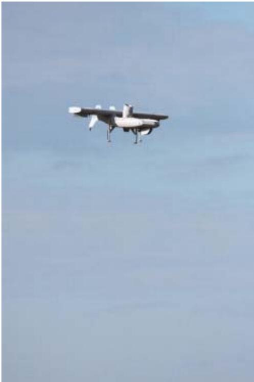
*Excalibur hovers on jet engine and electric lift-fan power during its June 24 first flight, which lasted just under 2 min. Takeoff, hover and landing were autonomous. Credit: AURORA FLIGHT SCIENCES CORPORATION/JOHN TYLKO*
