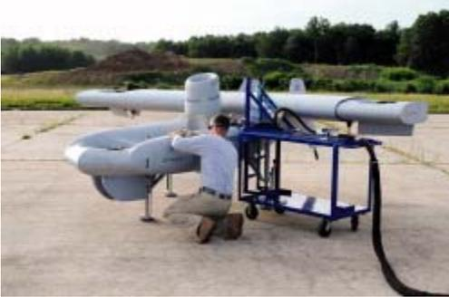
*The experimental unmanned combat aircraft is checked out before its first flight at Aberdeen Proving Grounds. Thrust-vectoring vanes under lift fans are used for yaw control. Credit: AURORA FLIGHT SCIENCES CORP./JOHN LANGFORD*
