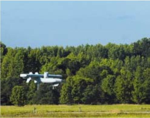
*Aurora plans to complete low-speed testing—“waking the box” in hover mode using the lift fans for attitude and speed control—on company funding. Credit: AURORA FLIGHT SCIENCES CORP./JOHN TYLKO*
