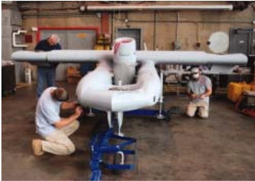
*Three 12-kw. battery-powered lift fans and a 700-lb.-thrust-class Williams F415 turbofan—developed to power the Tactical Tomahawk cruise missile—provide thrust for vertical flight. Credit: AURORA FLIGHT SCIENCES CORP./PATTI WOODSIDE*
